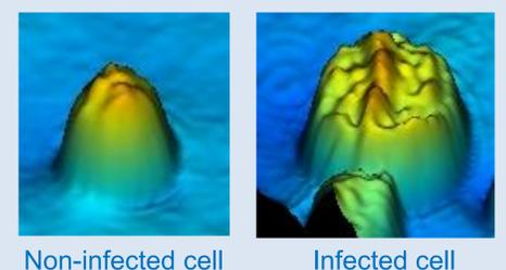
**Identification and count of blood cells:** each blood cell type has a particular optical fingerprint linked to its shape, size and content.
