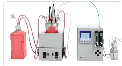
Figure 2: The iCELLis nano bioreactor system (from 0.53 to 4m<sup>2</sup>).
